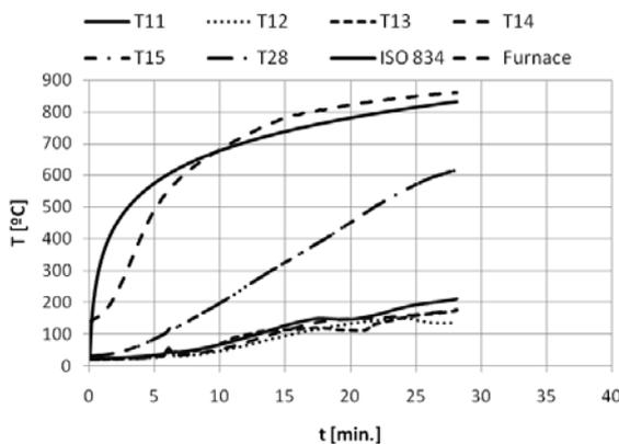
Figure 5. Temperatures in composite cross-section HEA160M
