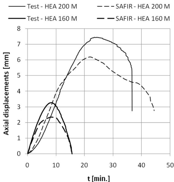
Figure 15. Axial displacements vs time for composite columns
