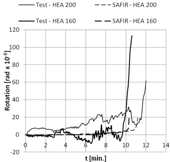
Figure 14. Rotations in top of the steel columns vs time
