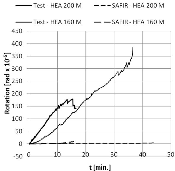
Figure 16. Rotations in top of the composite columns vs time
