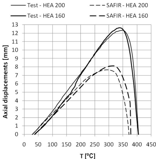
Figure 11. Axial displacements vs steel mean temperature for steel columns
