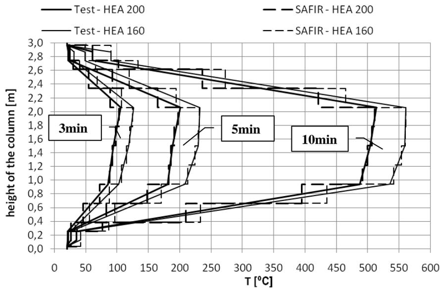
Figure 7. Distribution of temperatures in height for HEA160 and HEA200 steel columns
