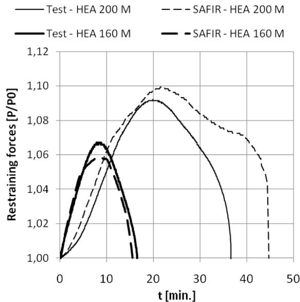
Figure 10. Restraining forces vs time for composite columns
