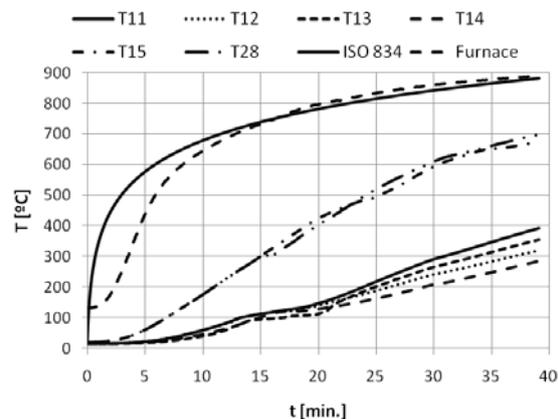
Figure 6. Temperatures in composite cross-section HEA200M
