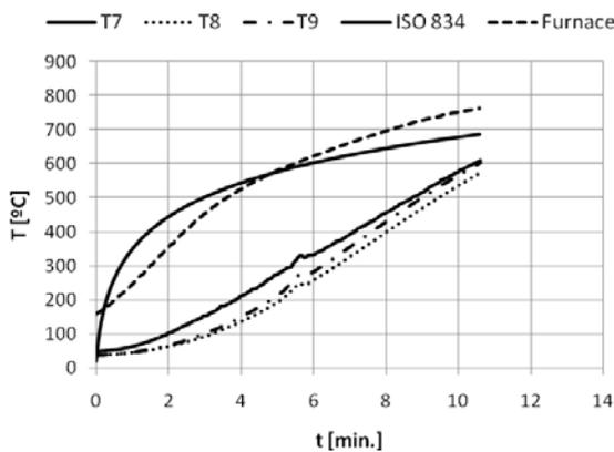
Figure 3. Temperatures in steel cross-section HEA160
