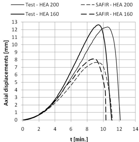
Figure 12. Axial displacements vs time for steel columns
