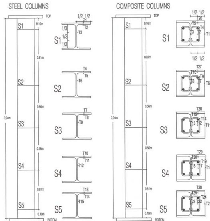
Figure 2. Location of thermocouples in the columns
