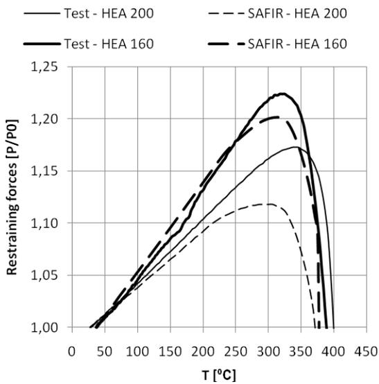
Figure 8. Restraining forces vs steel mean temperature for steel columns
