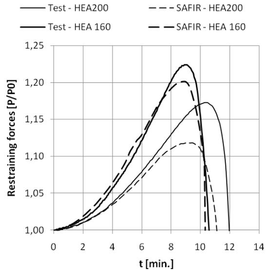
Figure 9. Restraining forces vs time for steel columns
