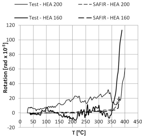
Figure 13. Rotations in top of the steel columns vs mean steel temperature
