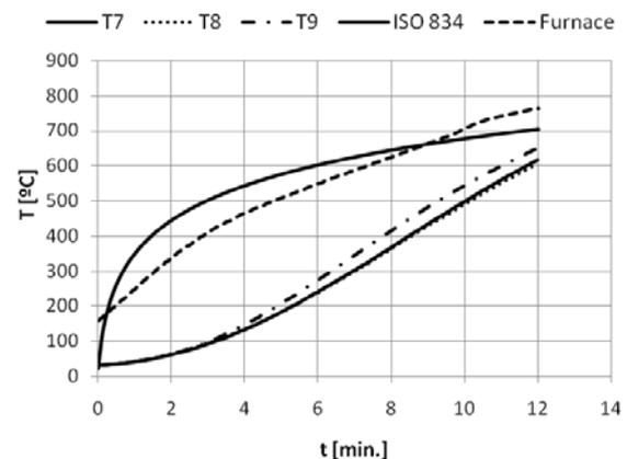
Figure 4. Temperatures in steel cross-section HEA200
