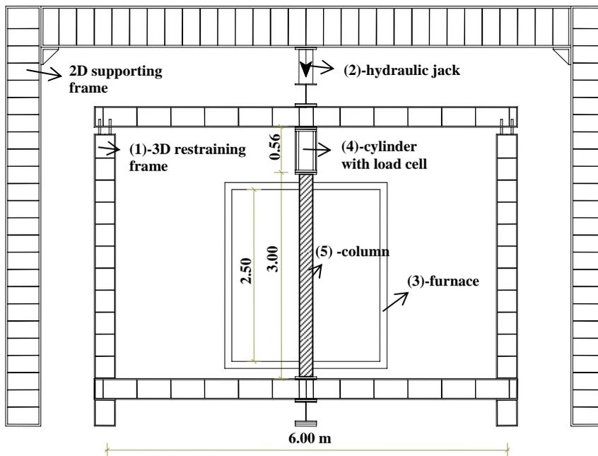
Figure 1. Scheme of the test set-up for fire resistance tests on columns
