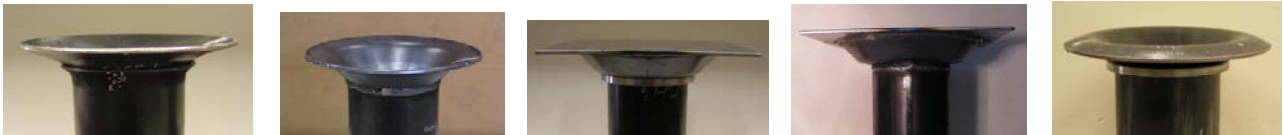
Figure 5. Failure deformation after test
