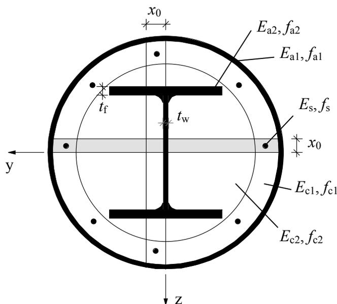
Figure 1 Cross section of a composite column in fire situation
