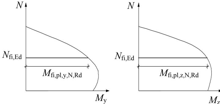
Figure 5 Design of compression and bending
