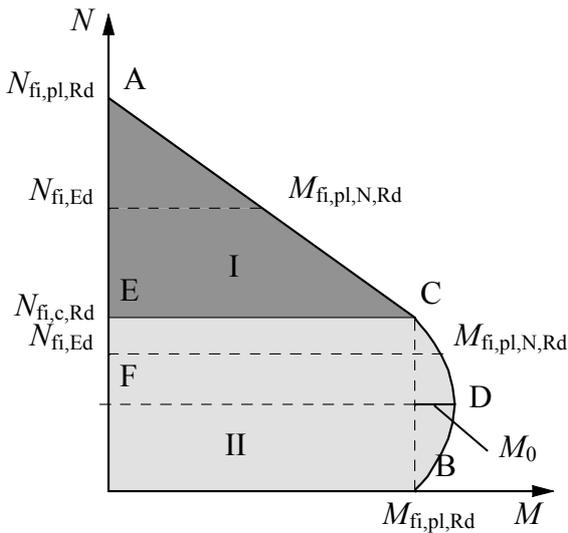
Figure 3 Simplified interaction curve for combined compression and uniaxial bending
