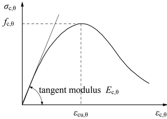
Figure 2 Stress-strain relationship for concrete in compression at elevated temperature  $\theta$
