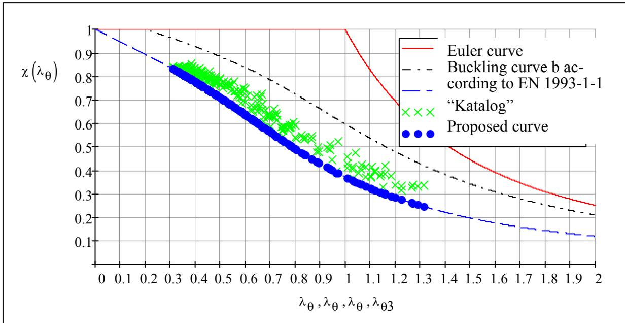
Figure 6 Comparison of “Verbundstützenkatalog” and the proposed buckling curve, see Viehl (2008)
