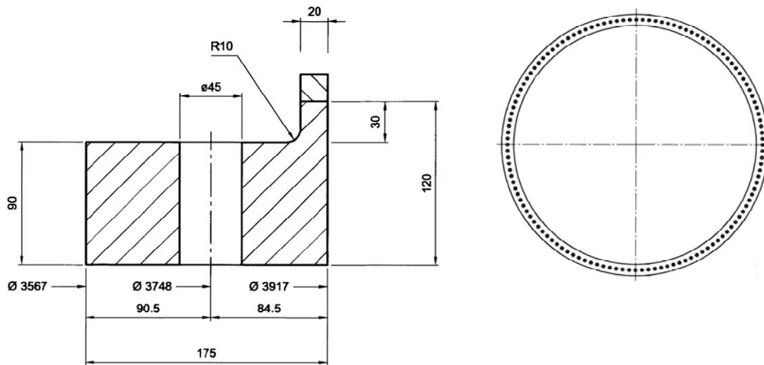
Figure 4. Dimensions and properties of the flange connection at section 1.
