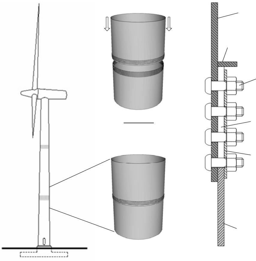
Figure 2. Principle of the proposed friction connection.
