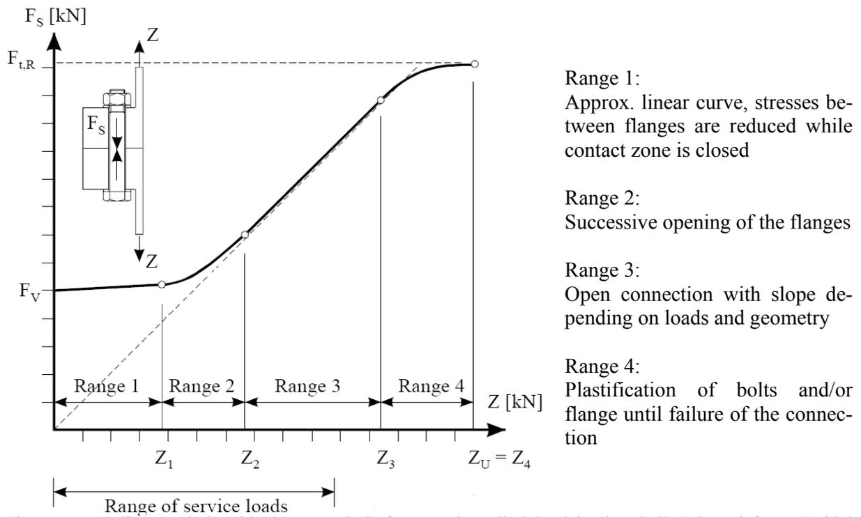
Figure 1. Nonlinear relationship between bolt force and applied load in the shell (adapted from (Seidel 2001b)).
