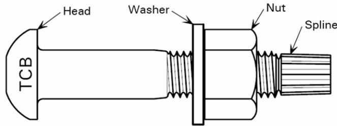
Figure 3. Tension Control Bolt, Grade S10T (Prior to pretensioning) (Cosgrove 2004).
