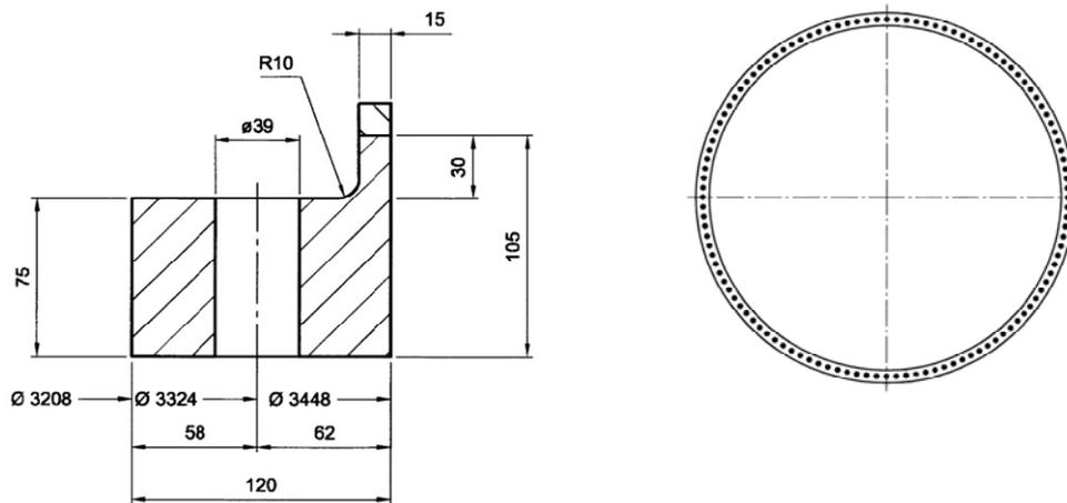
Figure 5. Dimensions and properties of the flange connection at section 2.
