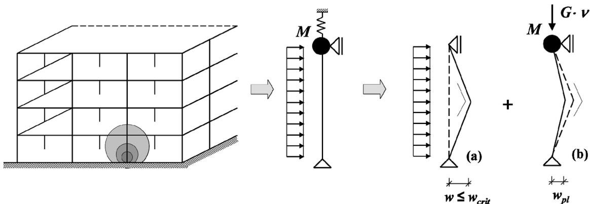
Figure 2. Design of structural member during (a) and after exceptional loading (b).
