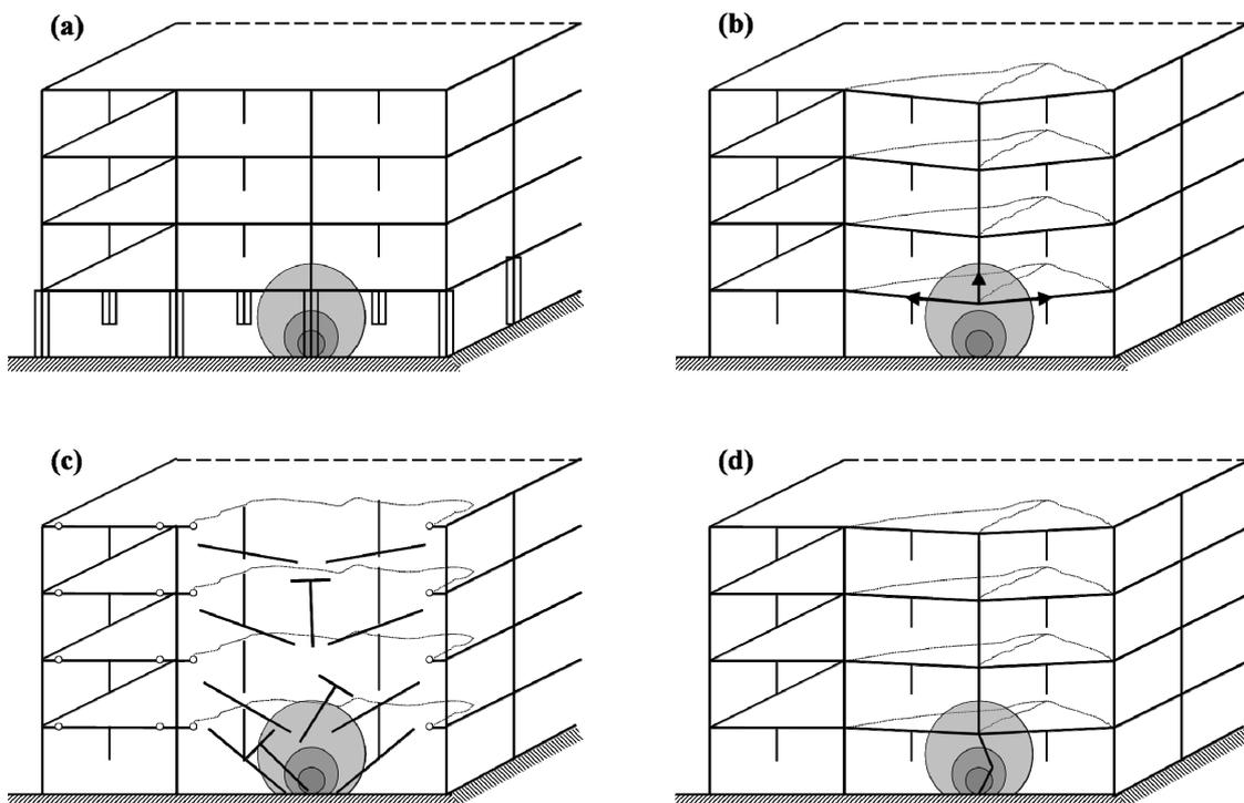
Figure 1. Strategies for robust structures: a) Key element method, b) Alternate load path method, c) Isolation of collapsed region, d) Residual strength method.
