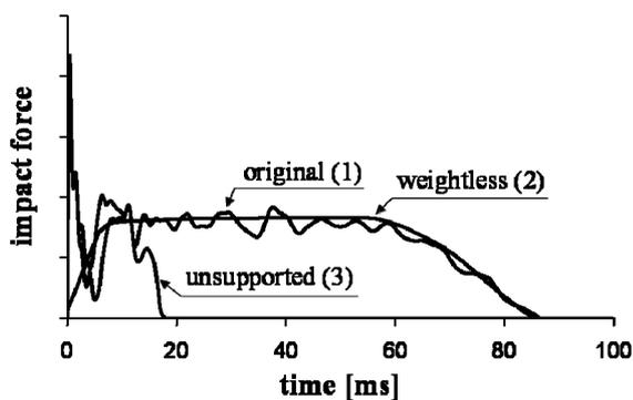
Figure 5. Impact force history for finite element models.
