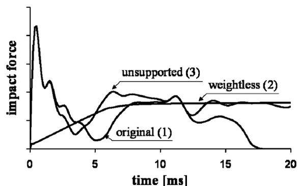
Figure 6. Impact force history for finite element models (close up).
