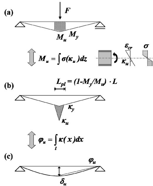
Figure 4. Analytical determination of the ultimate deflection.
