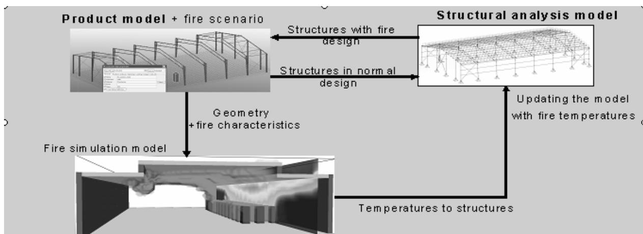
Figure 4. Natural Fire Design software combination.
