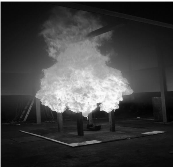
Figure 4. Freeburn test without sprinklers
