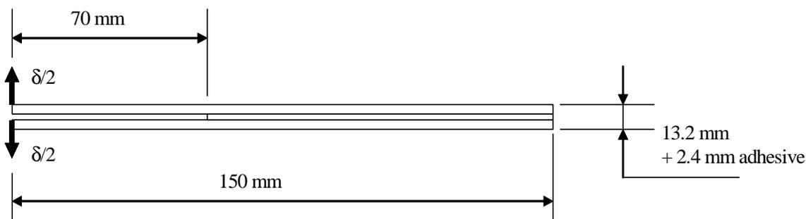
Figure 1. DCB, dimensions and geometry.
