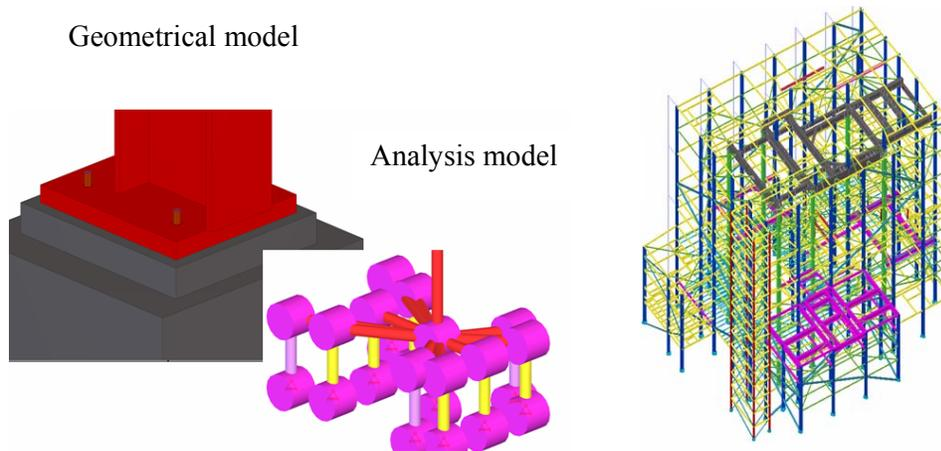
Figure 4. Industrial building skeleton and its base bolt models
