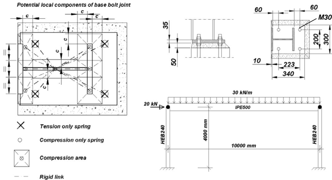
Figure 2. Potential local components, example joint and portal frame.
