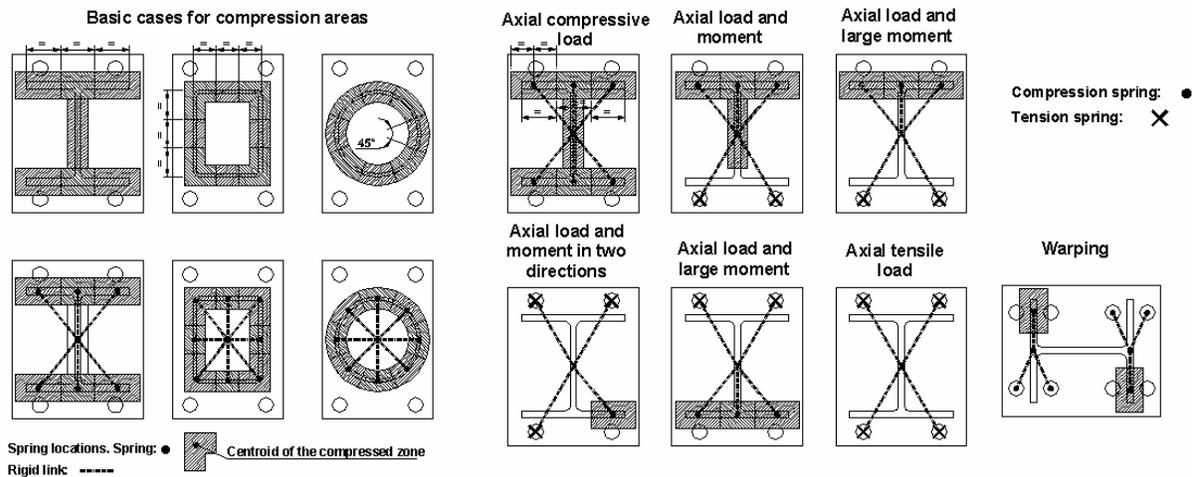
Figure 1. Examples of local analysis models for the base bolt joints.
