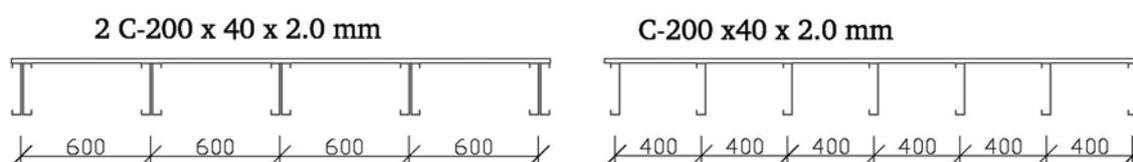
Figure 2. Configuration of the C-joists
