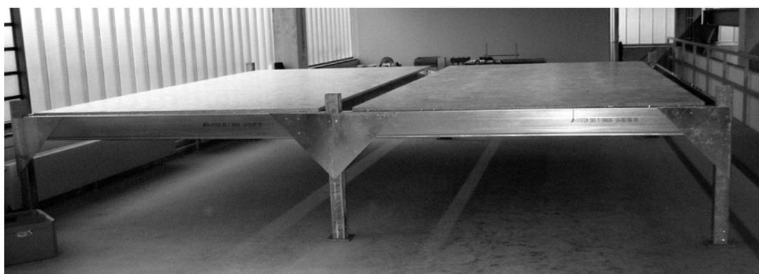
Figure 1. Test floors with C-joists and oriented-strand-board
