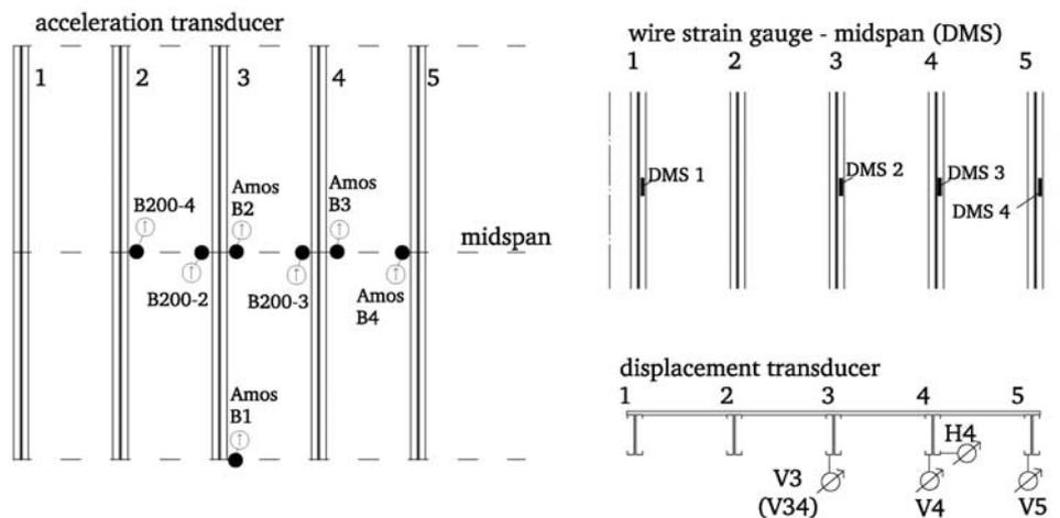
Figure 3. Configuration of the measurement technology
