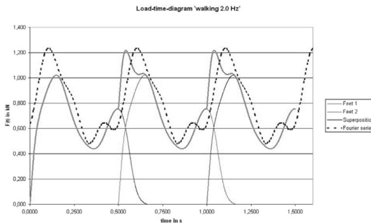
Figure 5. Load-time-diagram 'walking with 2.0 Hz'
