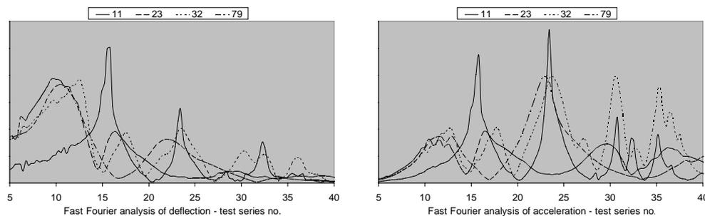
Figure 8. Natural frequencies by Fast Fourier Analysis
