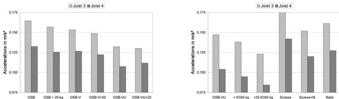
Figure 9. Comparison of accelerations  $a_{w,rms}$  of different stages of expansions - ‘Walking with 2 Hz’
