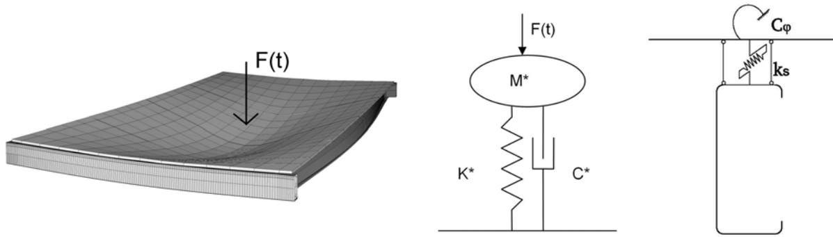
Figure 6. Equivalent static and dynamic system
