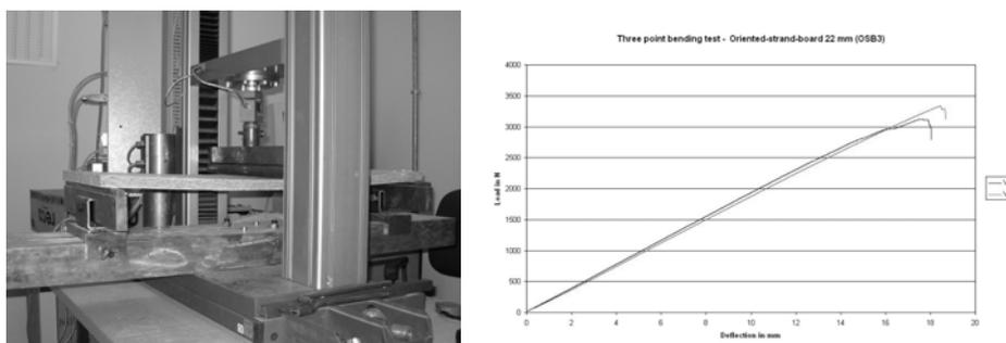
Figure 4. Three point bending test – Oriented-strand-board
