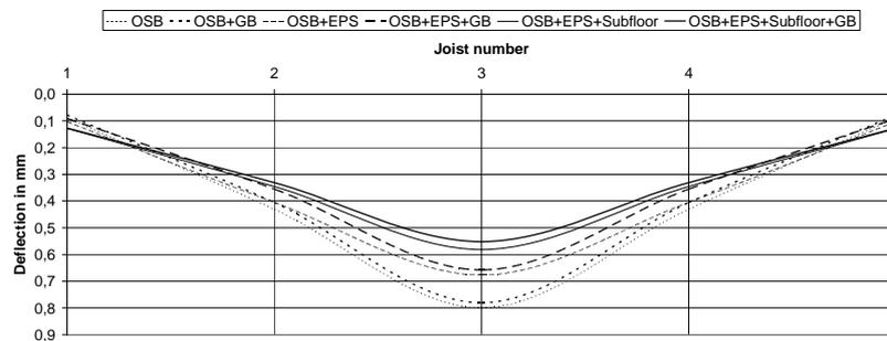
Figure 7. Midspan deflections (load sharing)
