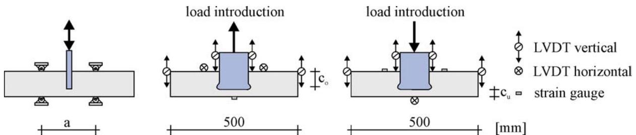
Figure 6. Bearing situation (left), Pull-Out Test (middle) and Push-Out Test (right).
