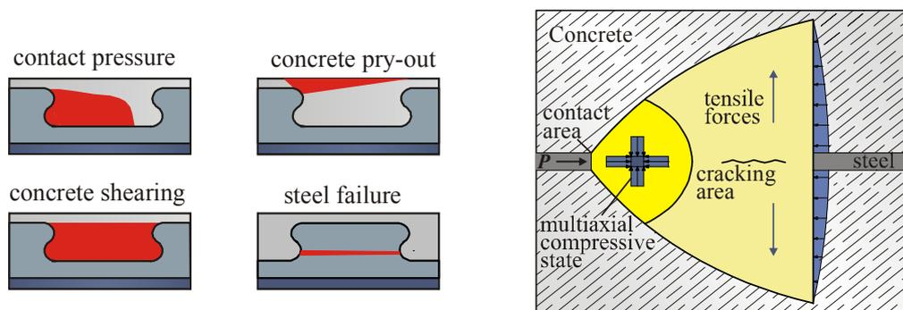
Figure 4. Failure modes (left) and stresses in the concrete (right) of continuous shear connectors
