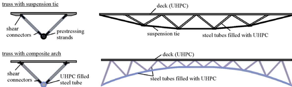
Figure 1. Hybrid Truss Beams
