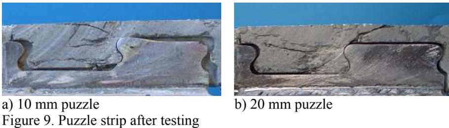
In the following, the results of the Single Push-Out Test (SPOT) are compared to the Push-Out Standard Test (POST) according to EC 4 (EC 4, 2004).
