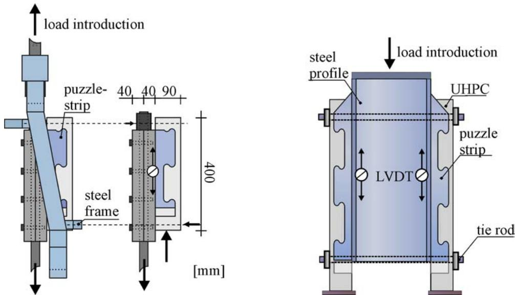
Figure 5. Single Push-Out Test (SPOT, left) and Push-Out Standard Test (POST, right).
