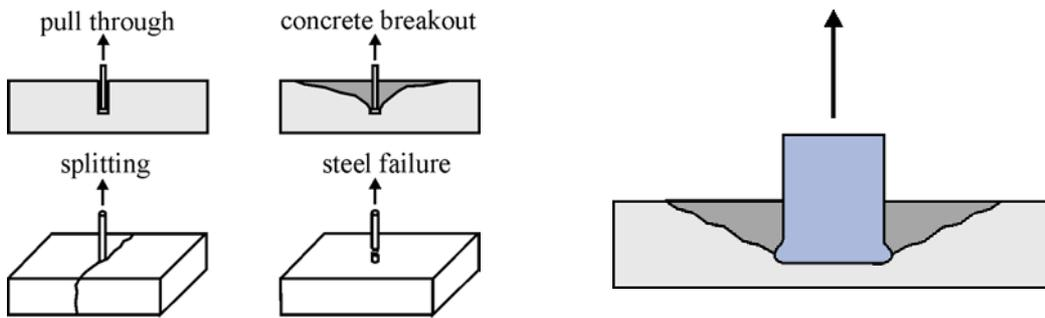
Figure 3. Types of failure (left) and concrete breakout of a puzzle tooth (right)
