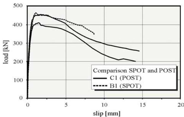
Figure 10. Comparison of POST and SPOT specimen (Series C).
