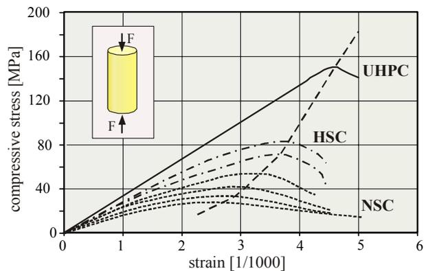
Figure 2. Characteristics of UHPC and stress-strain diagram
