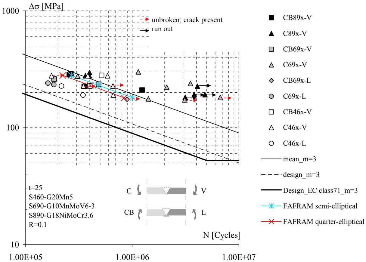
Figure 5. Fatigue strength curve of cracks initiating from the HAZ.
