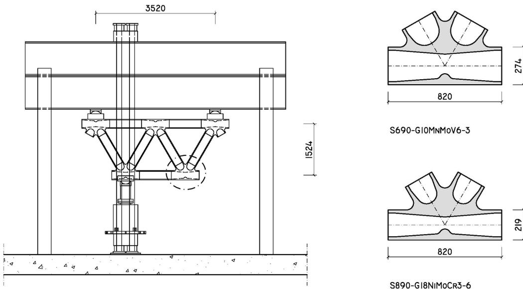
Figure 1. Conceptual drawing of large scale test setup for truss made of VHSS cast steel members and CHS.
