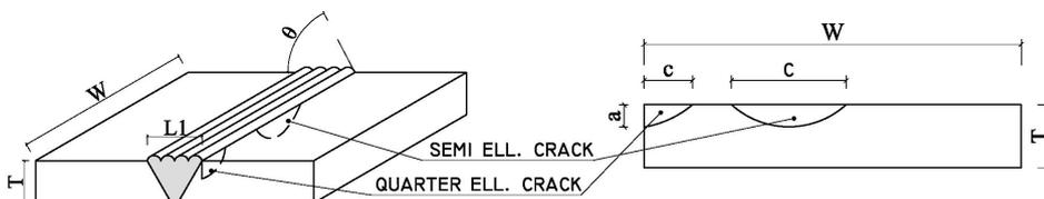
Figure 3. Geometrical parameters of V-welded hybrid connection.
