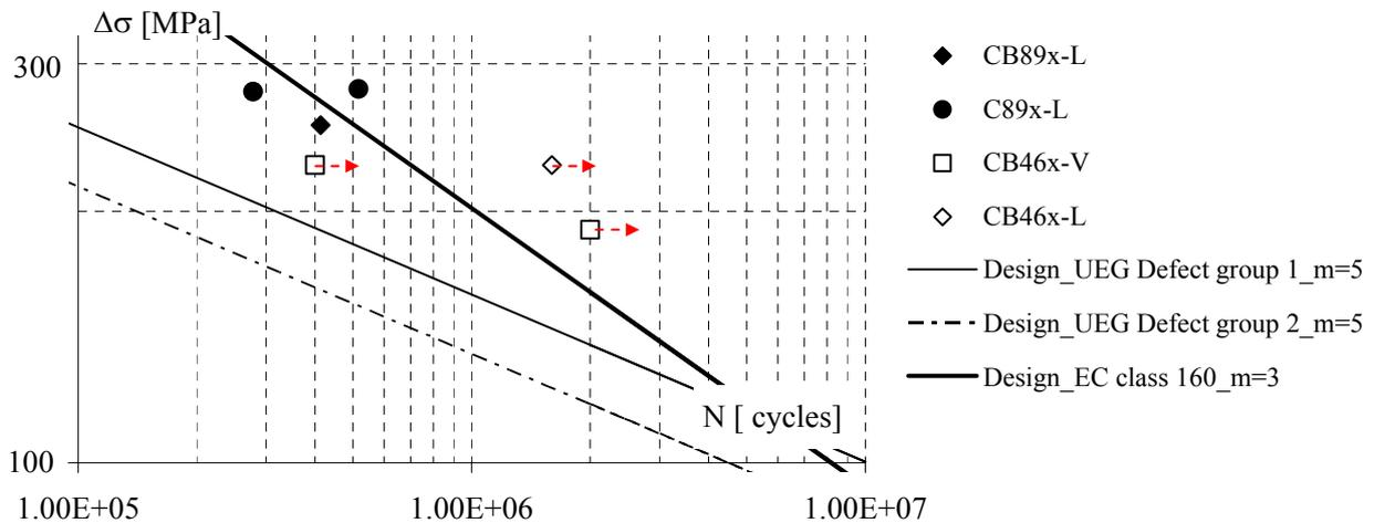
Figure 6. Fatigue strength curve of cracks initiating from base material.
