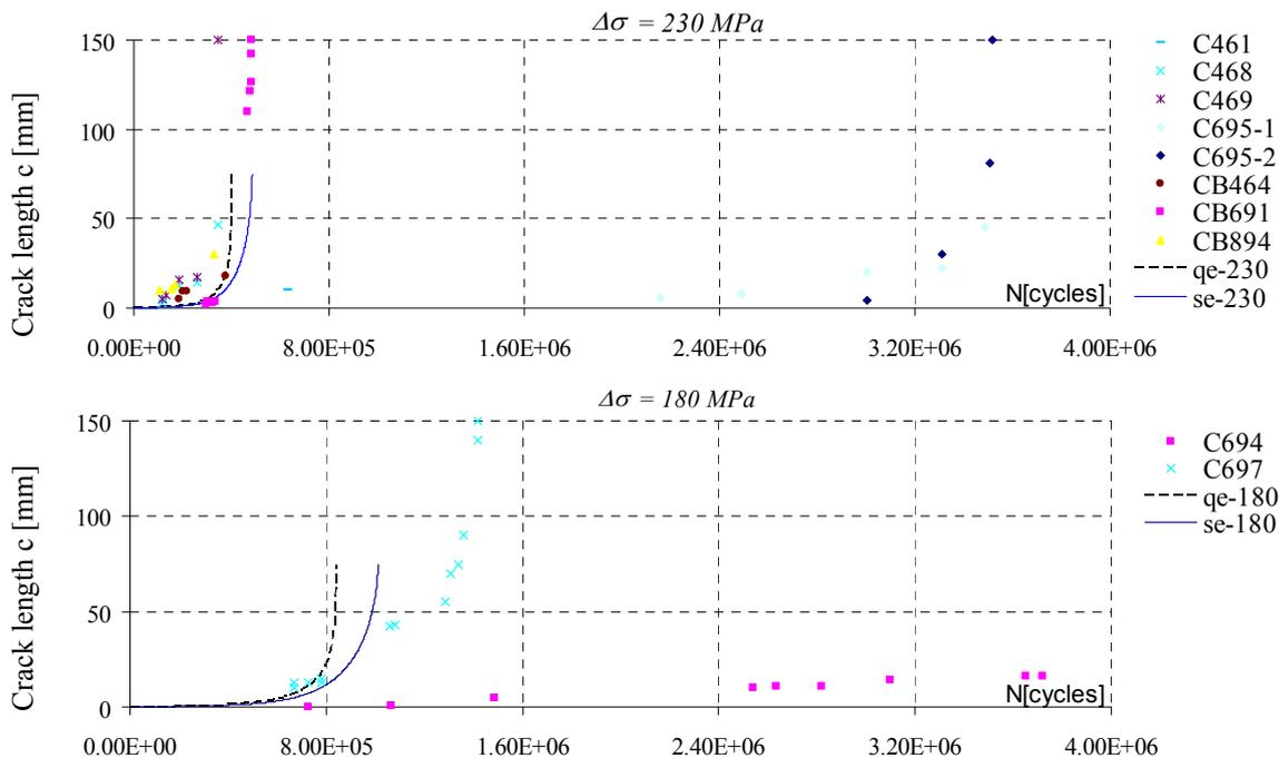
Figure 4b. Crack growth data.
