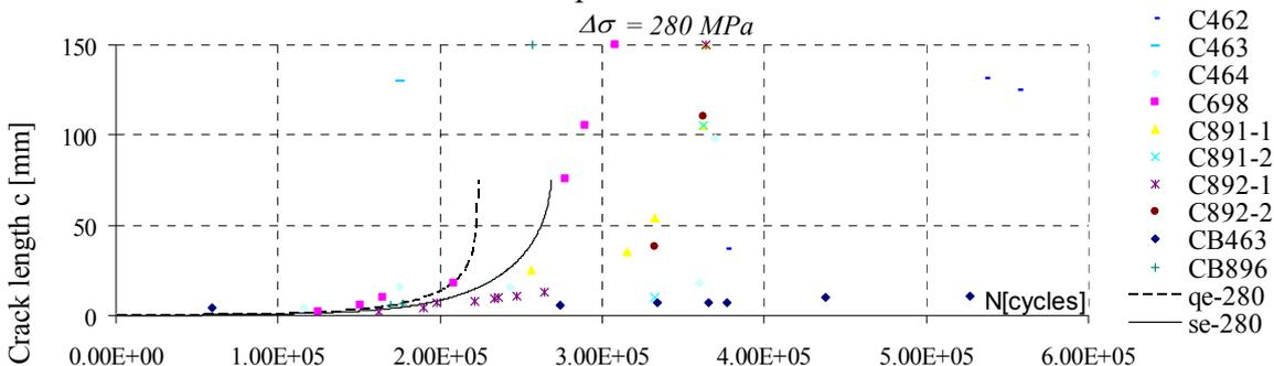
Figure 4a. Crack growth data.
