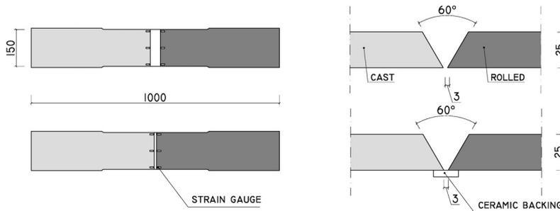
Figure 2. Geometry of small scale test specimens.
